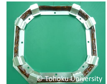
Magnetic Torquers (Electrical Coil)
