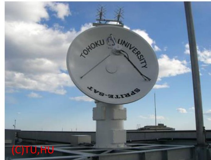
(C)TU,HU Dish-Antenna for S-Band
