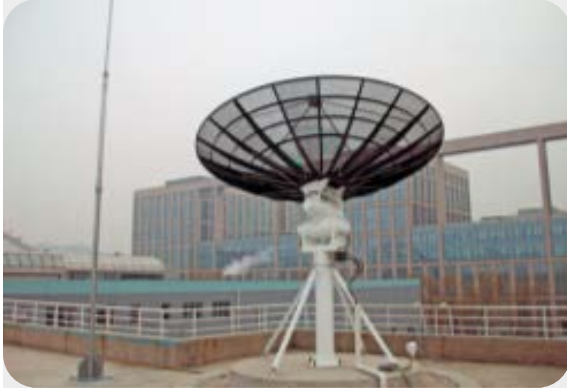
Ground Station for Remote Sensing Satellite Data Receiving
