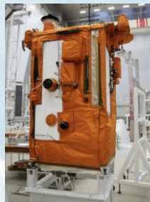
Vibro-dynamic testing of "AIST-2"
