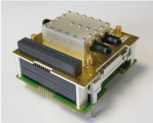
S-band transceiver with Diplexer (256/1000 kbit/s)
