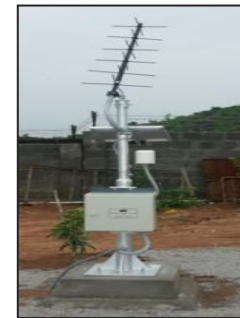
Automatic Weather Stations
