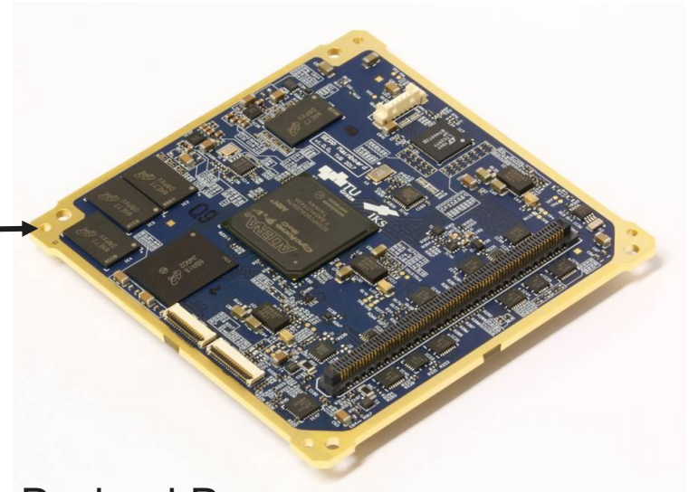
Payload Processor: System on Module Altera Cyclone V Memory 1 GB DDR3 RAM (ECC) 8 GB Industrial SD-Cards
