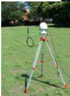
Radio for differential correction with base station
