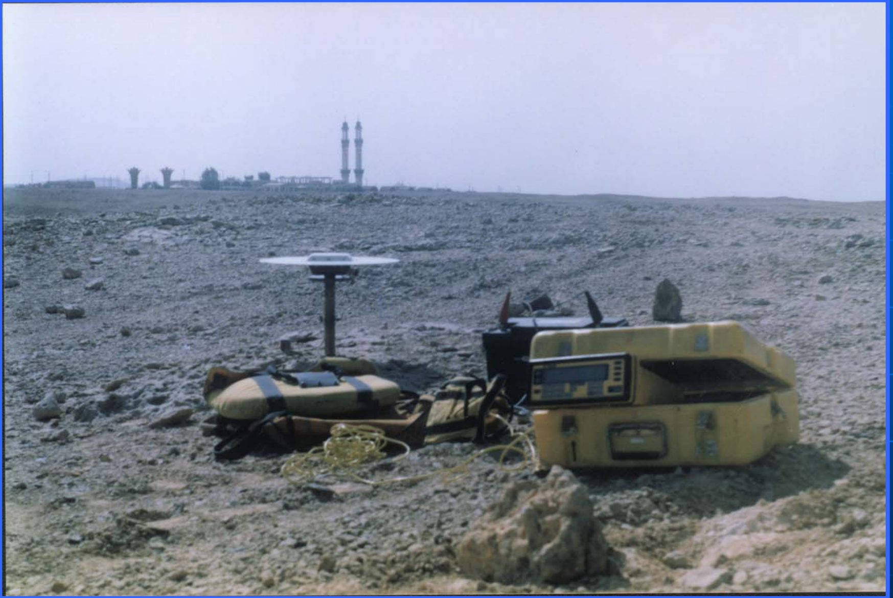
Survey Mode GPS Station: Antenna Connected with Trimble Receiver
