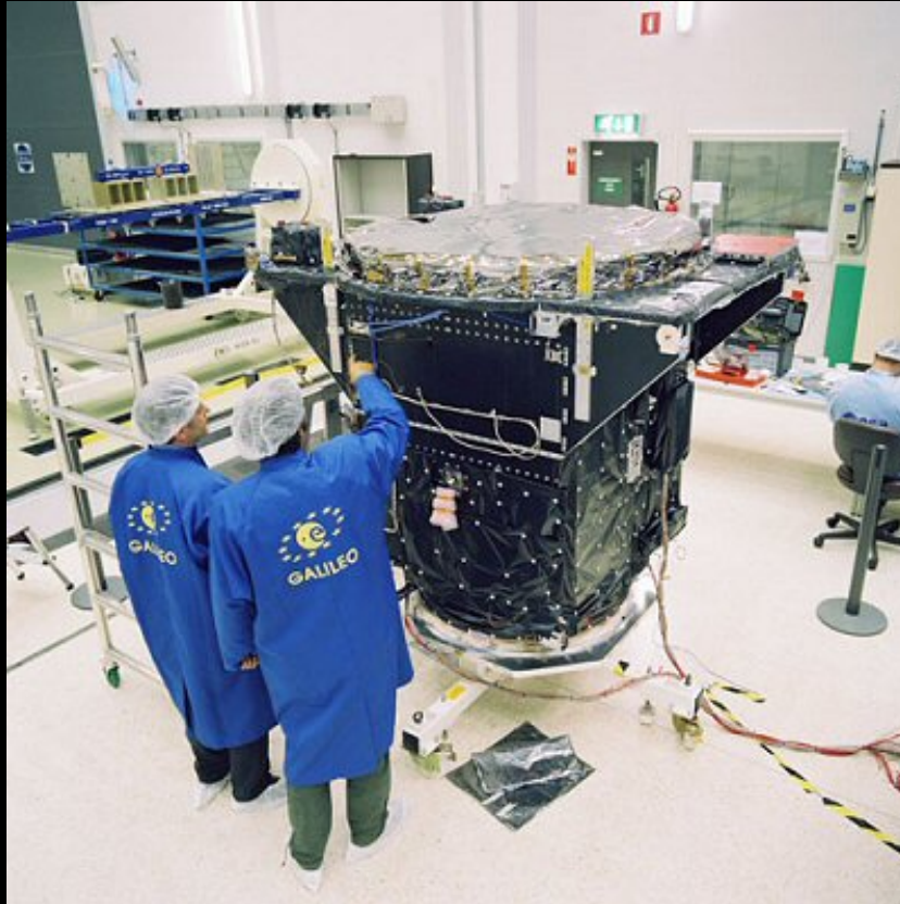
GSTB-v2 A satellite in the integration hall. The antenna is on the top face
