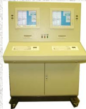
Maritime differential corrections station
