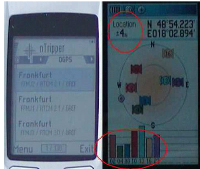
Without DGPS - precision of the position is +/- 4m.
