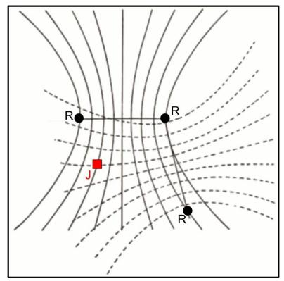
Three or more receivers with nanosecond-level time coordination can determine the location of a jammer by measuring time difference of arrival of the jammer signal
