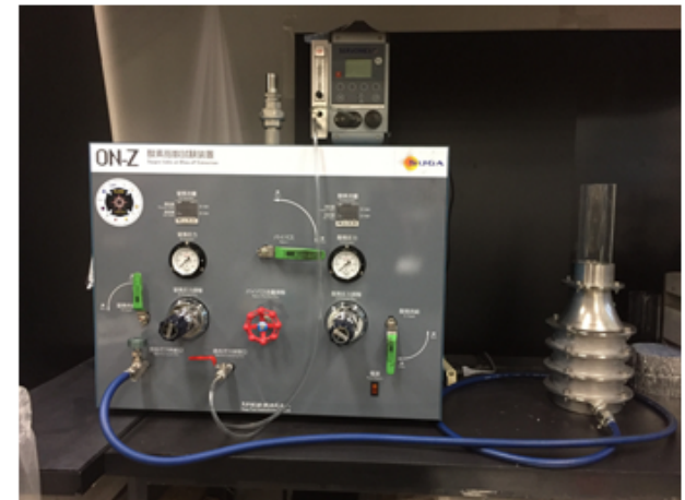
Set-up for the HOI method (ISO/DIS 4589-4).
