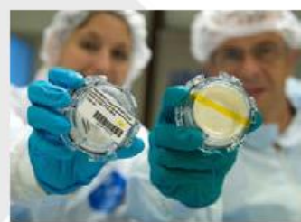
Aquapad: During the ISS Proxima mission, CNES, in partnership with the bioMérieux company, tested a technology to detect microbial contamination of water. The technology, which is simple and can be stored in ambient conditions, has been used on Earth for the detection of cholera in high-risk locations.
