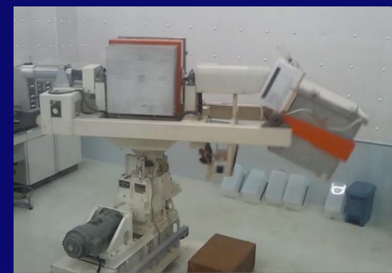
1.5m-radius centrifuge at Gifu University
