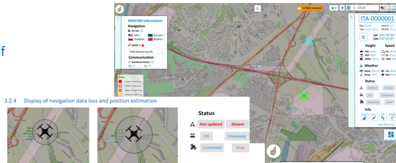
Figure 12: Display of the uncertainty sphere of a position in different time intervals: t=0 and t=1 sec
