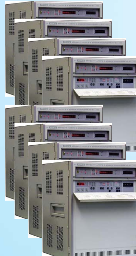
8 H-Maser clocks Kvarz CH1-75A \sigma_y(\tau) \leq 5 \text{ E-16} per day
