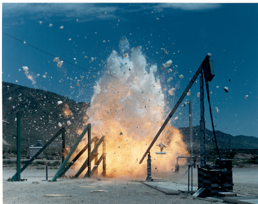
Figure 5: Liquid hydrogen liquid oxygen blast environment test
