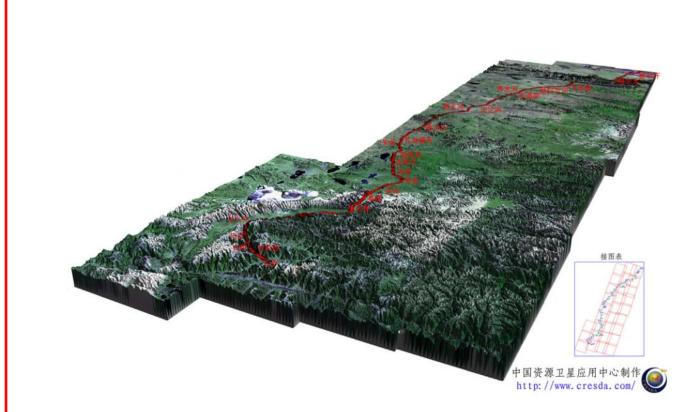
Three-dimensional image map for Qinghai-Tibet Railway, resulting from data of CBERS-2 CCD camera and 1:250000 DEM data
