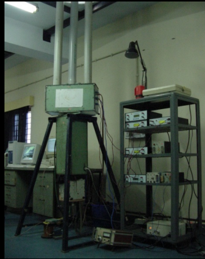
Multiwavelength dayglow photometer
