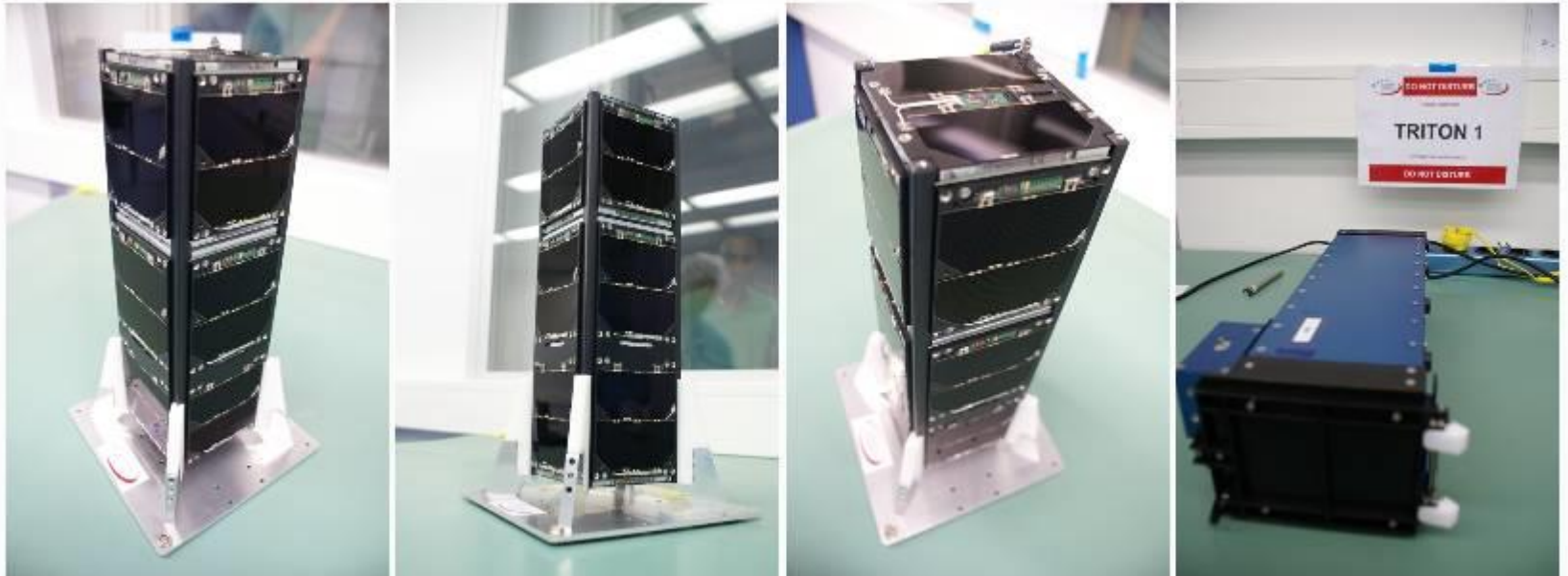
ISIS Triton 1 satellite with an on-board AIS receiver
