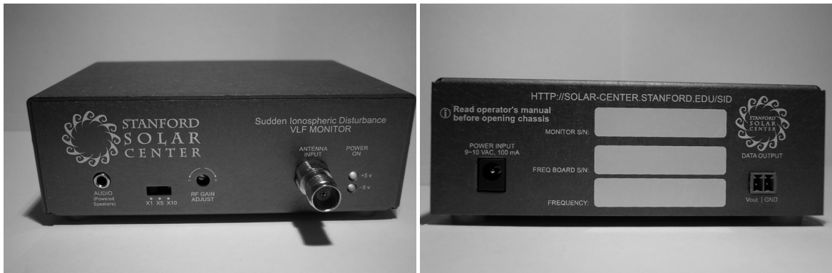
Figure 9. Front (left) and back (right) of the Stanford Solar Center SID monitor. Students assemble an antenna and provide an Internet connection to become part of a growing network of space weather monitors.
