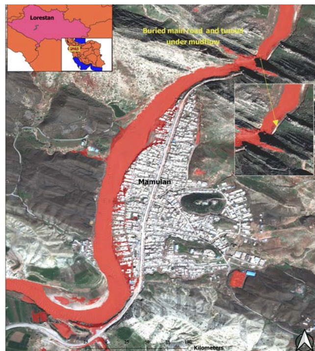
Inundation map of flash flooding produced by ISA as part of an activation of the International Charter "Space and Major Disasters" in 2019.
