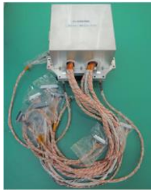
Power Control Computer
