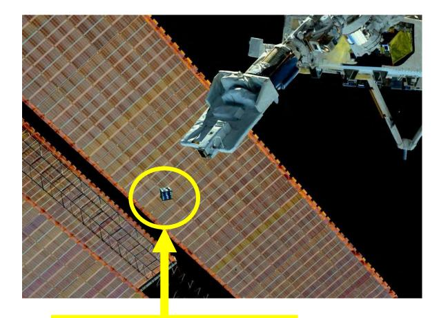
A 1U CubeSat being deployed from the ISS into low earth orbit
