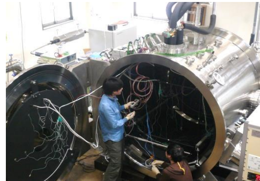
Thermal vacuum chamber at CeNT
