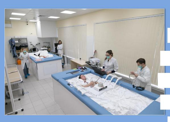
Ground-based microgravity model – Dry Immersion
