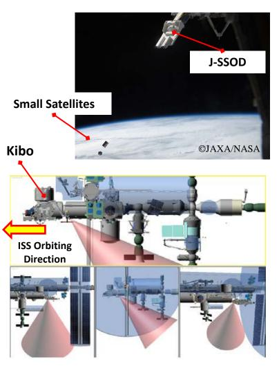
Deployment Direction(Cone) Nadir-aft 45° from the ISS nadir side
