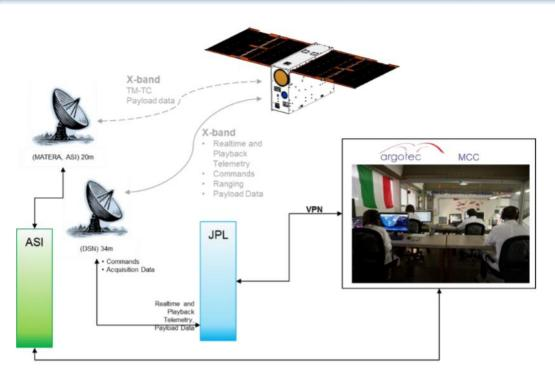
Communications based on X-band up and downlinks, with support of NASA DSN antennas and Italian facilities involvement, like the Sardinia Deep Space Antenna
