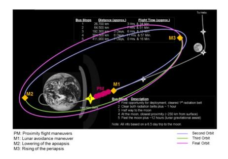
Orbital maneuvers will inject the cubesat into a geocentric orbit with high apogee, so allowing several moon flyby and imaging.
