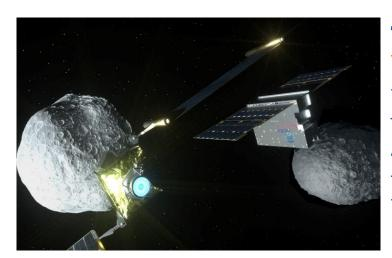
The Light Italian Cubesat for imaging of Asteroids - LICIACube will fly as piggyback of the NASA-APL DART probe towards the Didymos binary asteroid system, and will then be released to witness the impact effects of the American probe on the secondary Didymoon, in order to test trajectory deflection method by kinetic impact for Planetary Defense.
