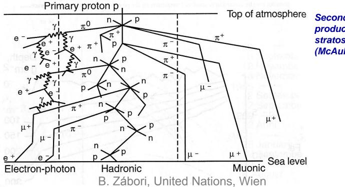
Secondary particle production in the stratosphere (McAulay et al., 1996)
