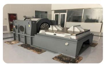
Thermal vacuum chamber 3.6m(Diameter)\*5.5m(Length) Thermal vacuum chamber 7m(Diameter)\*12m(Height) 200kN Shaker for Vibration Test
