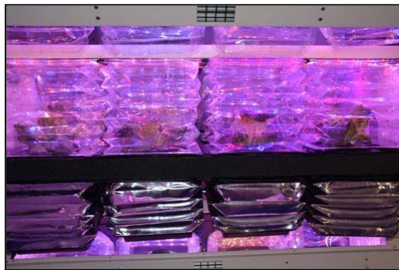
Plant Modules within GreenWall Section
