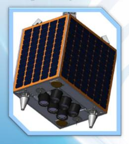
1. STSAT: technological space system ERS microsatellite (mass 110 kg), resolution 17 m Swath 300km.
