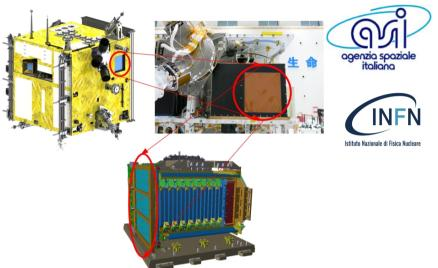
**Objectives:** Study of Litosphere-Ionosphere-Magnetosphere Coupling (LAIC), Solar Physics and Space Weather through concurrent measurements of 9 different instruments including an Italian particle detector (HEPD).
