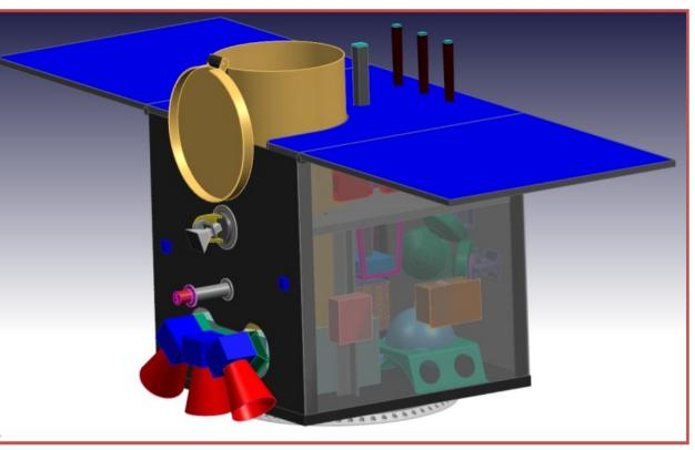
The NIR telescope is equipped with a panoramic interferometer based on a Fabry-Peròt etalon used in tandem configuration  $\rightarrow$  it combines high-spectral resolution with short exposure times
