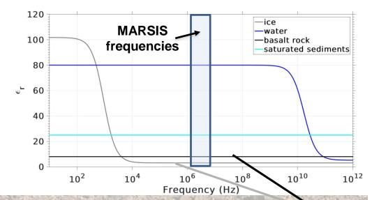
The capability to detect liquid water under the ice depends on the dielectric contrast between materials
