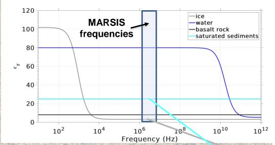
The capability to detect liquid water under the ice depends on the dielectric contrast between materials
