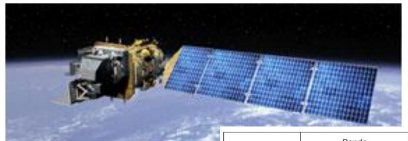
Landsat 8 Operational Land Imager (OLI) and Thermal Infrared Sensor (TIRS)
