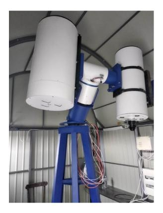
Twin tube (0.35 m f/2.0 and 0.25 m f/12) telescope with CMOS cameras has been installed in Transcarpathian region. It will be fully operational by the summer of 2022.
