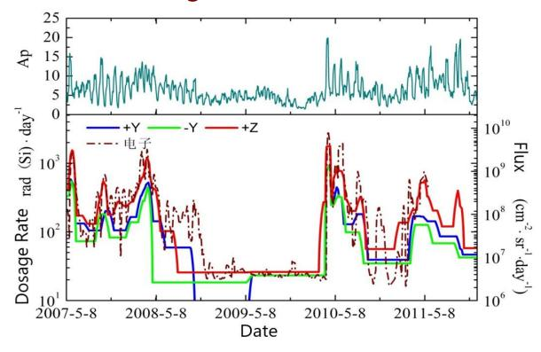
It can be seen that the radiation dosage is highly relative with the high energy electron flux, and modulated by the geomagnetic activities.
