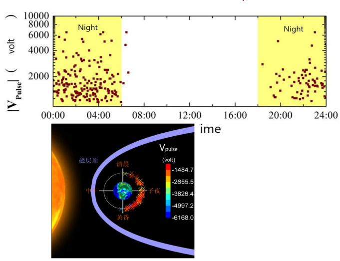
Most of the charge observations happened when the satellite locate at the night side of the magnetosphere, which indicates the charge phenomenon may be relative with the magnetotail plasma injection events.
