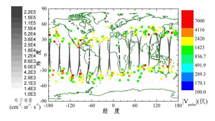
Pulse charge-discharge had been observed many times, which can charge the satellite surface to be thousands of volts in minutes.
