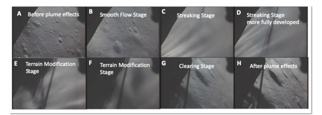
**Stages of rocket exhaust** ejecta beneath an Apollo Lunar Module. In smooth and streaking flow stages, ejecta is mainly in a sheet **1-3 degrees above horizontal**, although some individual streaks are at higher angles. In terrain modification stage much of the ejecta is lofted into higher angles **exceeding 15 degrees**.
