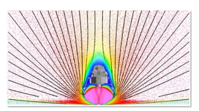
Apollo Lunar Module plume impingement at a distance of 5 m above the landing surface. Image shows plume gas velocity vectors colored by velocity magnitude (blue = low, magenta = high) as well as streamlines indicating the strong upward flow direction under vacuum conditions. **Credit: NASA**  Rocks and larger particles may directly damage equipment.
