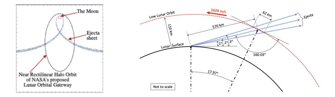
Left: Simulation of ejecta sheet traveling far from the Moon. Right: Geometry of Ejecta Flux Impacting a Spacecraft in Low Lunar Orbit.
