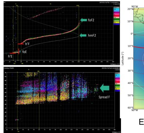
lonogram examples showing different parameters of the ionospheric layers, and the spread-F
