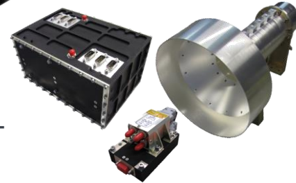
S-Band downlink system - Tesat Cooperation - (DDS)
