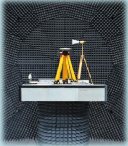
Tests of GNSS receivers and antennas
