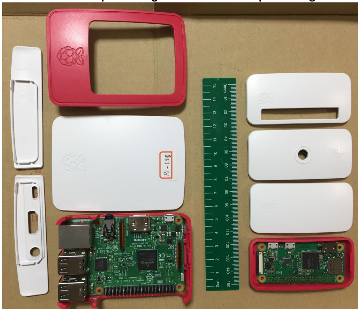
Raspberry Pi 3B for Realtime and Postprocessing RTK
