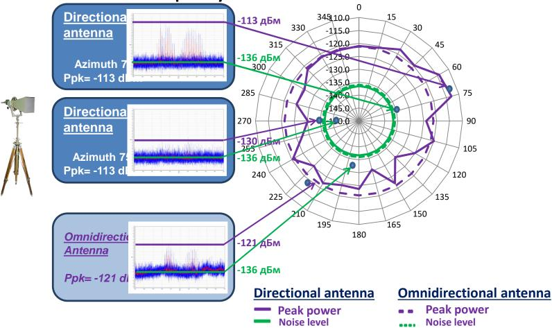
Crowdsourcing for Jammer Detection & Location (J911) Geographic Coverage Is the Challenge for IDM Systems; Detectable Range May Only Be a Few Hundred Feet and Multipath Effects Can Be Severe
