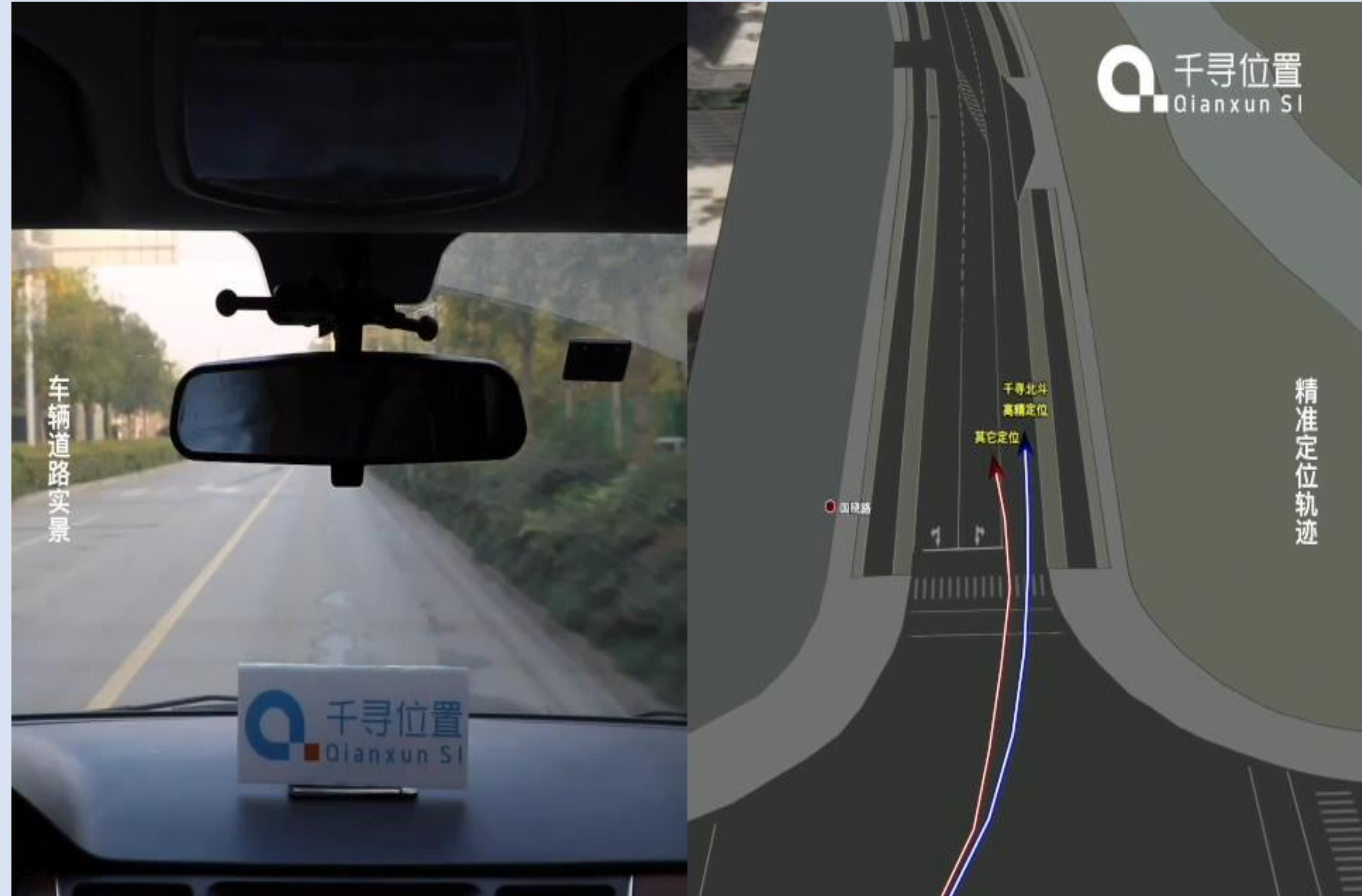
Lane level positioning on road test
