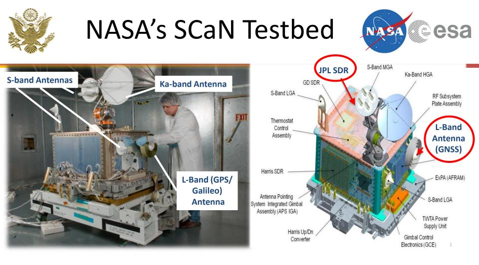
Space Communication and Navigation (SCaN) Testbed Installed on the Space Station in July 2012 Fully reprogrammable Software Defined Radio capability at L-band
