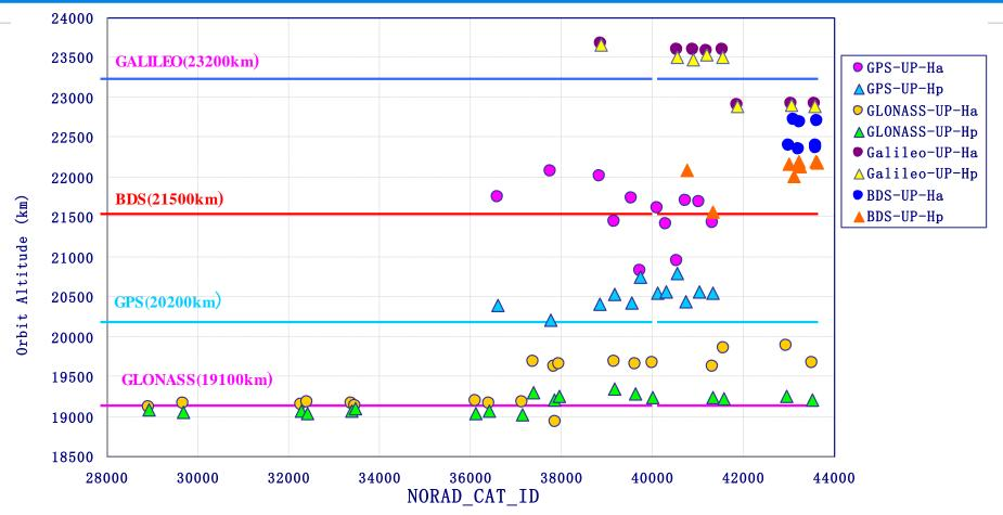
Most of the Upper-stage of GPS have crossed the BDS operational orbit, while two Upper-stages of Galileo is very close to the Upper-stage of BDS.Accordingly, we should also pay more attention to the safety of the GNSS Upper-stage.
