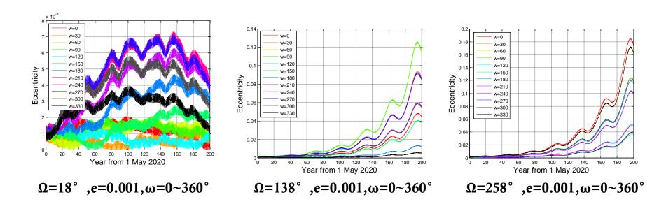
Recommendations for initial disposal orbit elements of BDS MEO satellites in the 1<sup>st</sup> plane:  $\triangle a_1 \ge +300$ km, $e_1 \le 0.001$ , $\omega_1 \ne 240$  ~270 °
