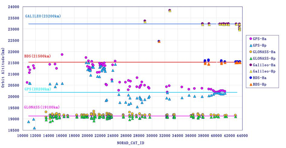
The post-mission satellites of GPS,Galileo and BDS have increase in orbit altitude, while Glonass satellites at the end of life stay in operational orbit.
