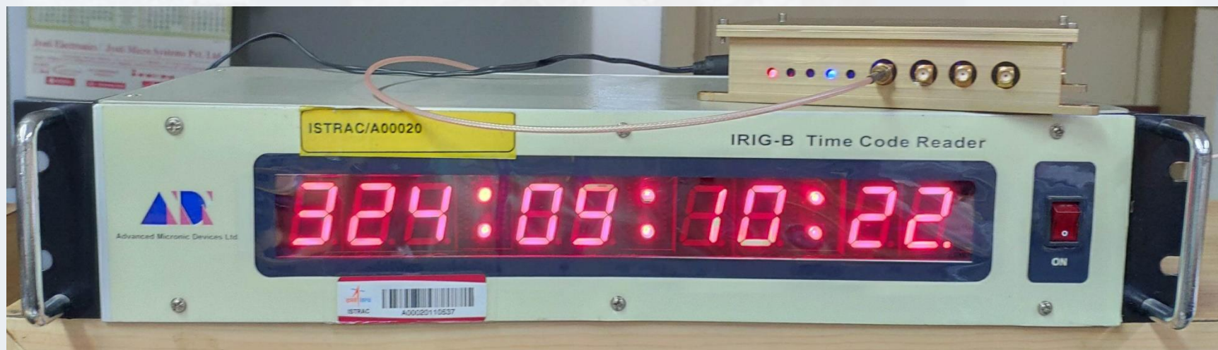
Receiver Timing output to standard IRIG B120 Time Code Reader
