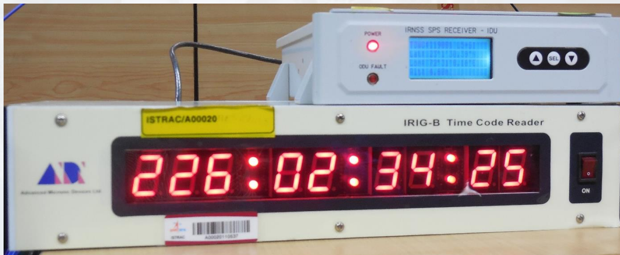
Receiver Timing output to Standard IRIG B120 Time Code Reader
