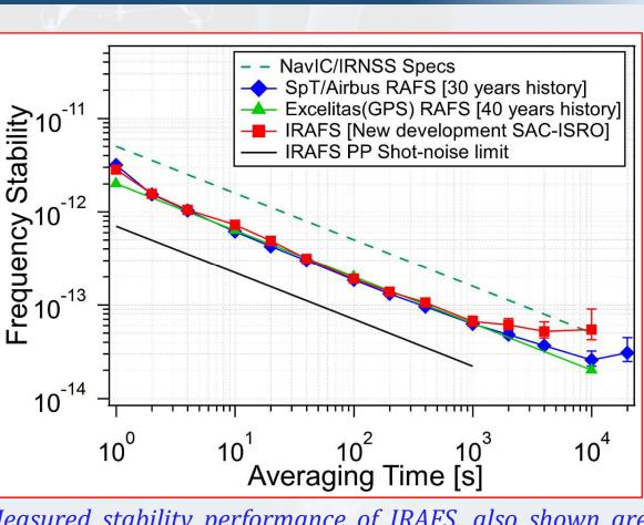
Power: <80 W (turn ON) <40 W (steady state) Weight: <10 kg (IRAFS+EPC) Measured stability performance of IRAFS, also shown are IRNSS specifications and shot-noise limit of the Physics Package.
