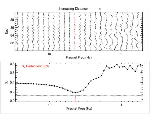
2. Geometric model provides Fresnel frequency vs distance. Intersection with measurement gives distance to irregularities.
